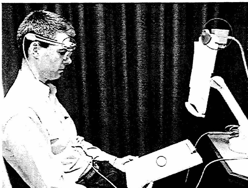
Figure 2: Transmitter and receiver cubes. In the configuration shown there is one transmitter cube shown on the stand to the right in the image (large circle) and two receiver cubes, one on the wearer's head attached to the trial-frame and one inside the clip board (small circles).
